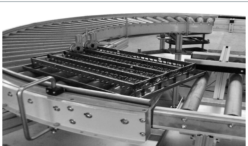
Curved roller track with conical rollers
