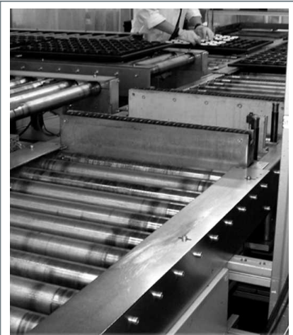
Lift/transverse unit with chain conveyor
