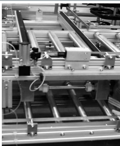
Lift/transverse unit with double belt conveyor
