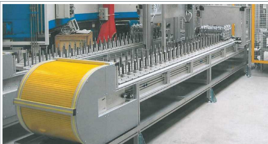
Horizontal accumulating conveyor / WPC transport Infeed of cast parts to machining cells
