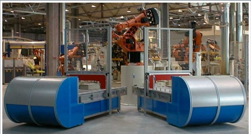
Horizontal accumulating conveyor / WPC transport Infeed of automotive body parts to a welding cell
