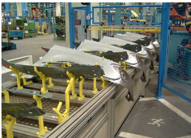
Horizontal indexing conveyor / WPC transport Infeed of automotive body parts to a welding cell
