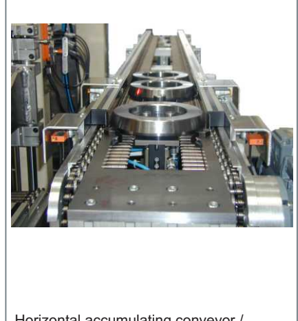
Horizontal accumulating conveyor / transport without WP carrier Infeed of unmachined parts for processing
